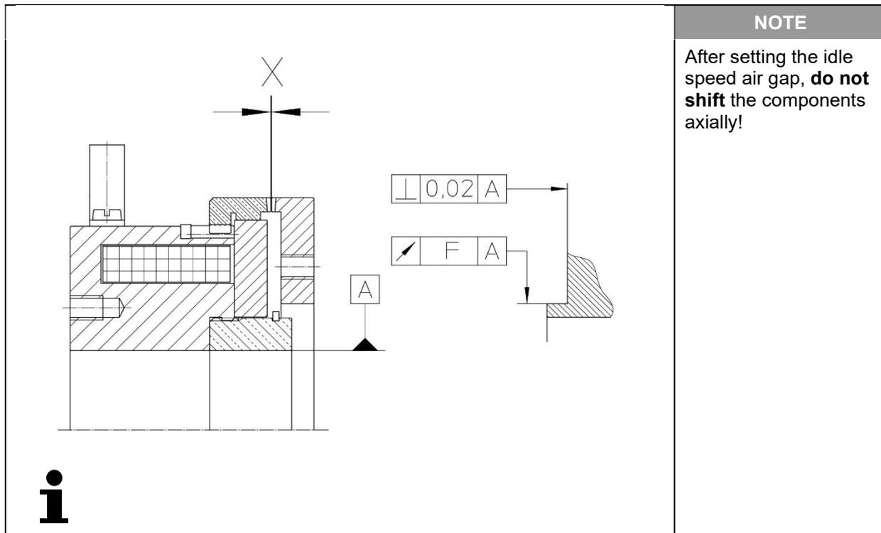
Figure 2: idle speed air gap "X"
